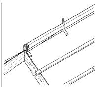
2. Fix galvanised ridge batten straps to each truss or rafter using clout nails. Using 25mm tiling battens make the ridge batten. For most tile profiles two to three battens will suffice. An extra batten may be necessary if a ridge board already exists. Secure the battens in place with ridge batten strap supplied overlapping the arms as necessary. Fix with clout head nails.
