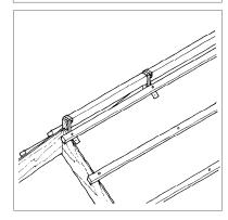
3. Fix the top tiling batten ensuring an air gap is maintained.
