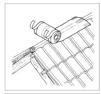
4. Unroll the TileLine Ridge Roll Ventilation System centrally over the ridge batten ensuring a 75mm overlap on each side of the top course of tiles. Secure in place every 300mm with clout nails or staples. Any joins should be overlapped by a minimum of 75mm.
