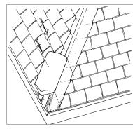
5. Using a 100mm screw provided secure the block end hip tile to the hip batten. (it may be necessary to drill a hole in the hip tile approximately 30-40mm from the block end for this purpose.)
