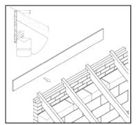
1. Fix a suitably sized ridge board to the end of the rafters. Check that the top of the board will be above the uppermost point of the finished height of the top course of tiles.
