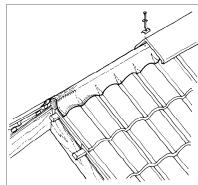
6. Locate the block end ridge tile over the centre of the roll and secure it with a screw (it may be necessary to drill a hole in the ridge approximately 30-40mm from the block end for this purpose.) Continue along the ridge fixing each ridge tile with the plates and screws provided.
