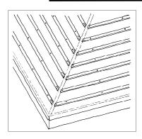
1. For unventilated dry hip applications, install the underlay as normal. For ventilated dry hip applications, lay the underlay and battens, cutting the underlay 30mm short of the hip on both sides of the hip to allow for ventilation. Ensure the ends of the battens are securely fixed where they meet the hip.
