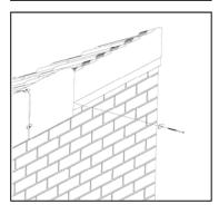
4. Remove the protective paper from the adhesive strip and press down firmly onto dry, clean tiles all the way along the ridge. For deeply profiled tiles, additional care is needed to work the TileLine Ridge Roll Ventilation System into the pans.
