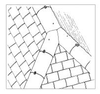
6. At the apex close mitre the hip and ridge tiles, drill and secure to the hip and ridge batten using the 100mm screws provided. If the TileLine Ridge Roll Ventilation System is not used on the ridge continue the roll 200mm onto the ridge in place of the standard lead saddle detail.
