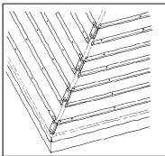
2. Hip batten supports in 50mm x 50mm timber should be screw fixed at the eaves and apex and spaced along the line of the hip rafter in between the tiling batten spaces as shown. Supports could be constructed from 2 x 25mm tiling battens.
