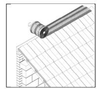
3. Unroll the TileLine Ridge Roll Ventilation System over the ridge board ensuring a 75mm overlap onto the tip course of tiles. Secure in place onto the ridge board every 300mm with clout nails or staples. Any joins should be overlapped by a minimum of 75mm
