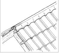
5. Remove protective paper from the adhesive strip and press down firmly onto dry, clean tiles all the way along the ridge. For deeply profiled tiles, additional care is needed to work the TileLine Ridge Roll Ventilation System into the pans.
