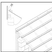
2. Lay the underlay in the normal way, but ensure that any fixings are set back at least 30mm from the inside face of the ridge board and there is sufficient free edge on the underlay to enable it to be wrapped onto the top batten.
