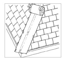
4. Working from the eaves, secure the TileLine Ridge Roll Ventilation System in place centrally over the hip batten using corrosion resistant nails or staples. Roll out along the hip batten and fix at 300mm centres. Remove protective paper from the adhesive strip and press down firmly onto dry, clean tiles all the way up both sides of the hip.
