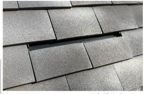
This is a discreet ventilator flush with the roof, designed to blend in to the rest of the roof tiles. Sections of Dreadnought tiles are bonded to the leading edge of the tilevent in the same colour as the tiles on the rest of the roof to match in.
