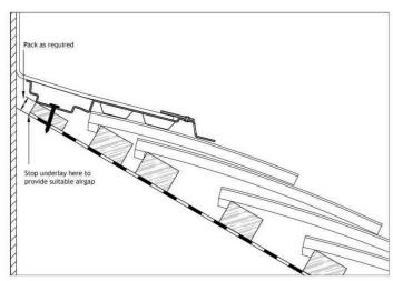
Starting at the edge of the roof, position the first Abutment Vent so its edge is level with the edge of the tile.
