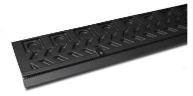
Prior to installation, check a suitable air gap and supporting batten for the Abutment Vent is present between the top course of tiles and wall. You may need to add some additional packing to support and secure the Vent.
