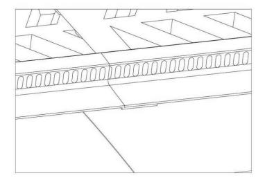
Bring down the flashing from the wall on to the top face of the Abutment Vent, terminating it behind the ridge of the forming above the ventilation grille. Tuck the flashing behind the pre-fitted clips to help prevent the lead lifting. Ensure the wall flashing covers the open ends of the vent to prevent insect and weather ingress.
