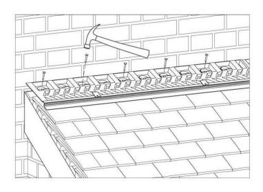
Moving left to right, fit the subsequent Abutment Vent by butting it to the fitted vent and repeating the fitting sequence until the full top abutment of the roof is completed. The last Abutment Vent will most likely need to be cut to ensure it finishes flush with the edge of the tiles.
